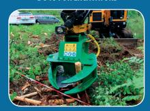
FARMA also offers BC 18 energy cutter to be used on excavators. Felling, gathering, cutting and loading everything from trees and brush to bushes and stumps can be easily handled. Trees are easy to cut and the fixed blade is easy to maintain. The location of the centre of gravity makes it easy to position the grapple directly by the root. The product is to be considered a combined grapple and felling
