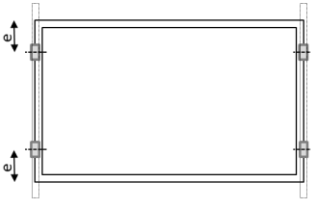
Fig. A2: Clamp position on short frames Mounting rails parallel to the shorter frame
