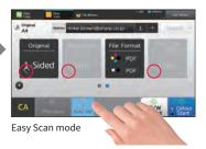
Automated settings that match the document The MFD can tell whether a document being scanned is colour or B/W. If it is B/W it can automatically select the optimal setting for text-monochrome or greyscale.
