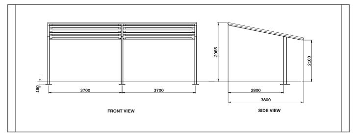
Dimensions (mm): Overall: 3300D x 2985H Internal: 2800D x 2100H Module length: 3700
