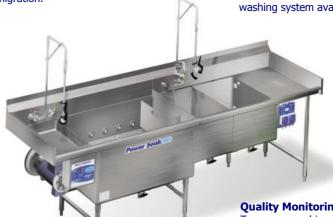
**Quality Monitoring** (P2 Controller Only) To ensure washing quality, Power Soak is programmed to have an LED light indicate when a water change is required. At set intervals, the water change feature disables the wash pump, forcing employees to empty the wash tank and refill it before the pump will resume operation. A separate light reminds employees when a water change is recommended for the sanitize
