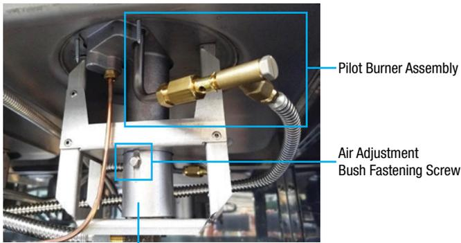
Fig.6. Air Adjustment Bush
