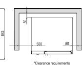
\*Clearance requirements \*Drain line must be vented
