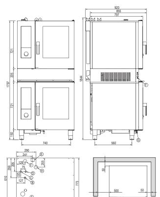
Heat Source: 500mm clearance from an external heat source is required in order to protect the oven control components and allow access to the service panel. For clearances under 500mm, it is mandatory for Stoddart heat shields to be fitted while still maintaining a minimum clearance of 300mm to provide access to the service compartment. Failure to adhere to minimum clearances may void the oven warranty or add service costs due to lack of access.
