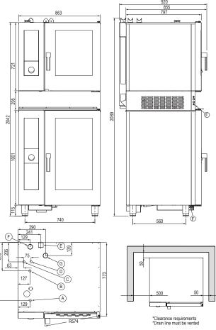
Heat Source: 500mm clearance from an external heat source is required in order to protect the oven control components and allow access to the service panel. For clearances under 500mm, it is mandatory for Stoddart heat shields to be fitted while still maintaining a minimum clearance of 300mm to provide access to the service compartment. Failure to adhere to minimum clearances may void the oven warranty or add service costs due to lack of access.
