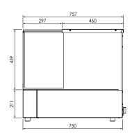
W.HFHSQ24 Model 1460 x 757 x 696 W x D x H (mm)
