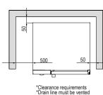
Heat Source: 500mm clearance from an external heat source is required in order to protect the oven control components and allow access to the service panel. For clearances under 500mm, it is mandatory for Stoddart heat shields to be fitted while still maintaining a minimum clearance of 300mm to provide access to the service compartment. Failure to adhere to minimum clearances may void the oven warranty or add service costs due to lack of access.
