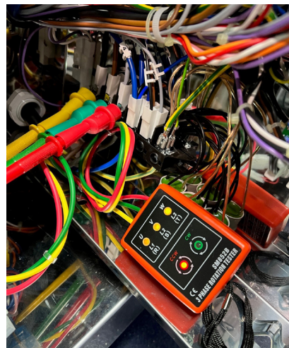
Phase rotation meter connected to supply terminal, accessed through front of unit
