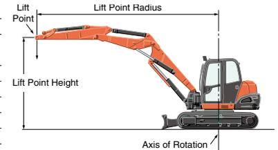
\* Working ranges are with Kubota standard bucket, without quick coupler.
