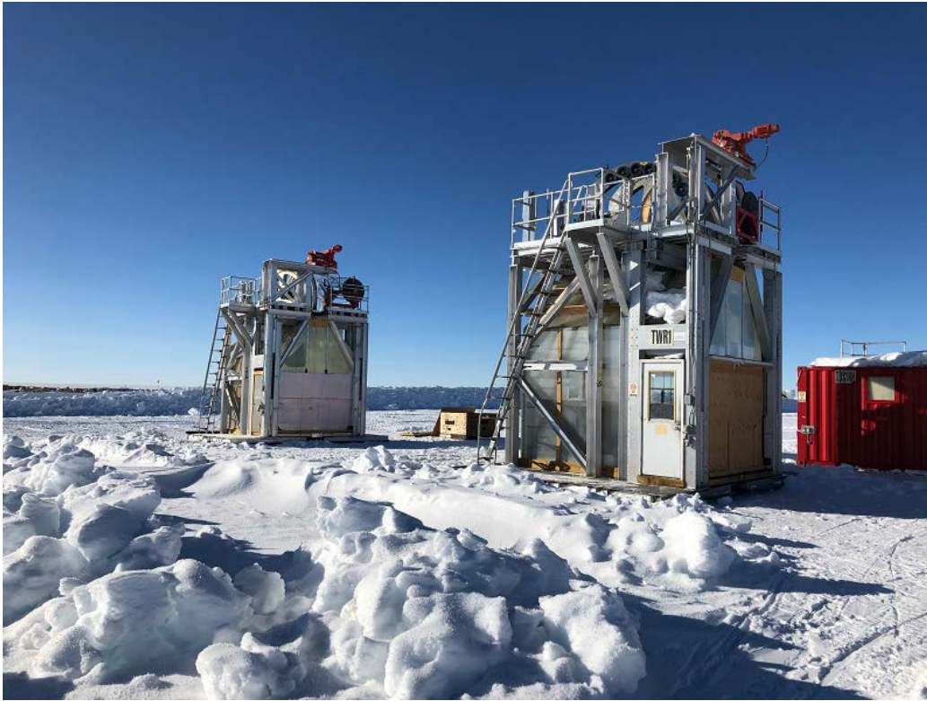
Figure 21: Towers 1 and 2 are shown from Gen1 operations. For Gen2, the towers will be on top of an Air Ride Cargo Sled and no longer on the snow.
