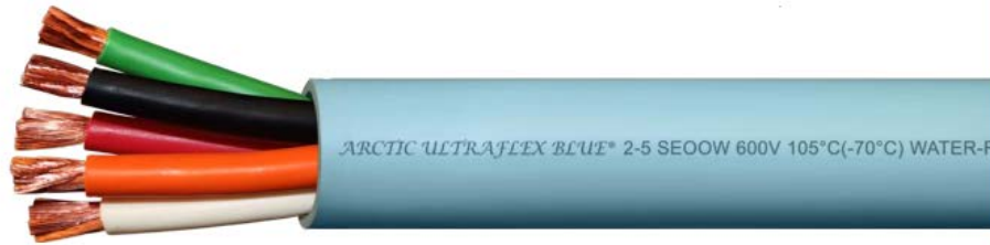
Figure 10: Arctic Ultraflex Blue® power distribution cable rated at 64 amps with five stranded 2 AWG conductors and a nominal outside diameter of 35 mm.
