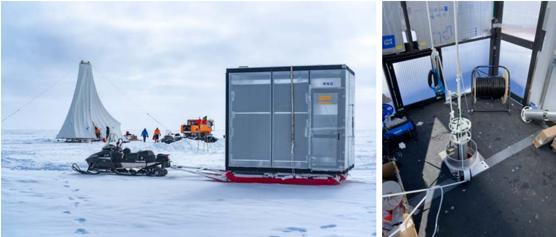
Figure 39: Deployment shack being positioned on top of a finished hole, while the next station hole is being drilled (left); antenna being lowered inside the shack (right).
