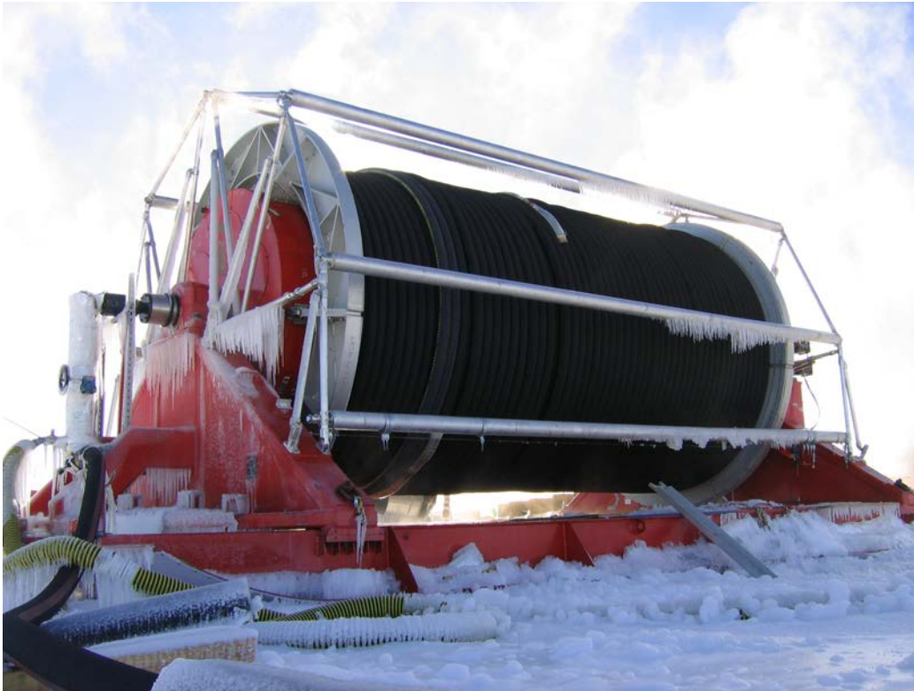
Figure 25: The Drill Supply Hose Reel from Gen1 and the IceCube Upgrade will be repurposed for IceCube Gen2.
