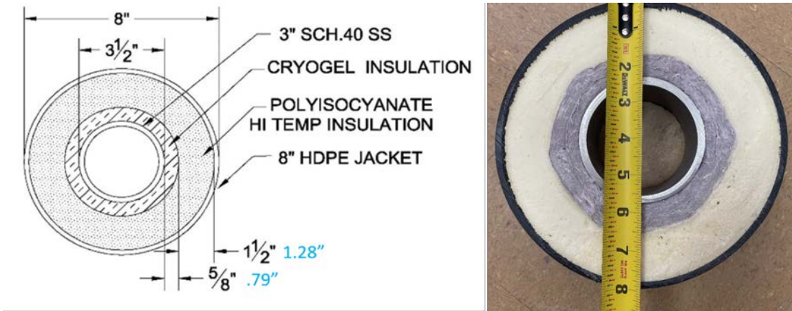
Figure 17: Left: Cross section of insulated Rovanco pipe. Differences in Tricon dimensions are shown in blue. Right: Sample of a cross section of insulated pipe. This sample features the polyisocyanurate insulation and a layer of pyrogel (cryogel/aerogel), which is another form of insulation.
