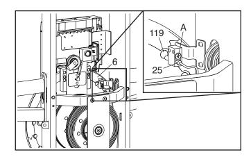
Then, rotate the Resistance Disc (6) until a Magnet (119) is aligned with the Reed Switch (25). Slide the Reed Switch slightly toward or away from the Magnet. Then, retighten the screw (A).
