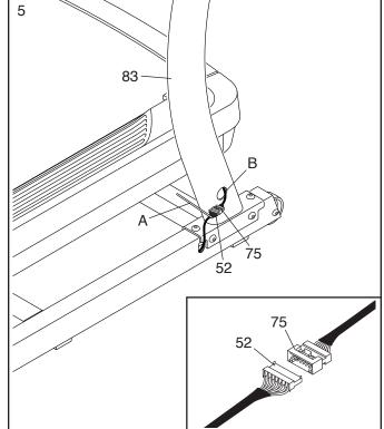
Identify the right handrail assembly (C). With the help of a second person, set the right handrail assembly on the console assembly (D).
