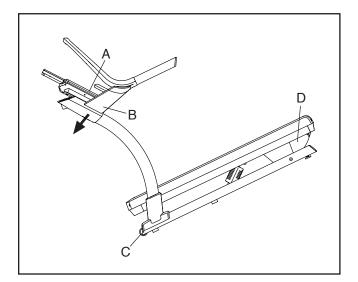
Carefully roll the incline trainer on the wheels to the desired location, and then lower it to the level position. CAUTION: To reduce the risk of injury, use extreme caution while moving the incline trainer. Do not attempt to move the incline trainer over uneven surfaces.
