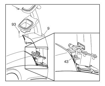
Next, tighten the indicated M8 Locknut (43) slightly to tighten the Drive Belt (not shown). Then, reattach the Front Shield Cover (9) and plug in the power adapter.
