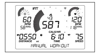
Calories (flame icon)—When the manual mode is selected, this display will show the approximate number of calories you have burned. When an onboard workout is selected, this display will show either the approximate number of calories remaining to be burned or the approximate number of calories you have burned.
