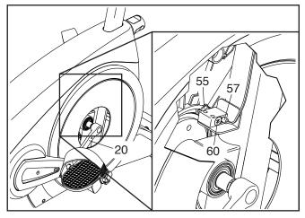
Plug in the power adapter and rotate the Left Crank Arm (20) for a moment. Repeat these actions until the console displays correct feedback.
