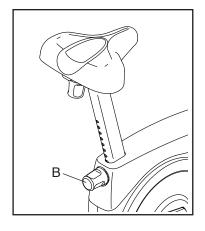
is engaged in one of the adjustment holes in the seat post. Then, turn the knob clockwise to tighten it.
