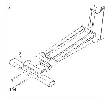
With the help of a second person, place some of the packing materials (not shown) under the front of the Frame (1). Have the second person hold the Frame to prevent it from tipping while you complete this step.
