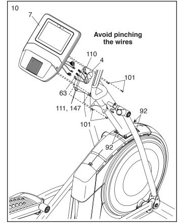
11. Orient the Rear Console Cover (80) as shown, and attach it to the Upright (4) with two M4 x 16mm Screws (101).
