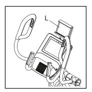
pivot the tablet holder to the desired position. Reverse these actions to remove the tablet from the tablet holder.
