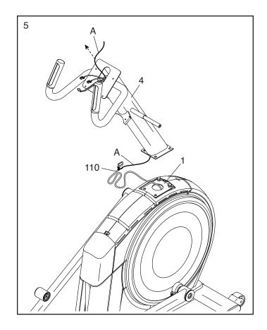
6. **Tip: Avoid pinching the Main Wire (110).** Have a second person hold the Upright (4) on the Frame (1).
