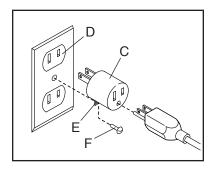
The lug (E) or wire extending from the adapter must be connected with a metal screw (F) to a permanent ground such as a properly grounded outlet box cover. Some 2-pole receptacle outlet box covers are not grounded. Before using an adapter, contact a qualified electrician to determine whether the outlet box cover is grounded before using an adapter. The temporary adapter should be used only until a properly grounded outlet can be installed by a qualified electrician.
