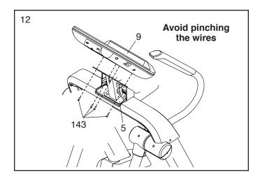
13. **Tip: Avoid pinching the wires.** Attach the Console Bracket Cover (48) to the Accessory Tray (111) with two M4 x 16mm Screws (143).
