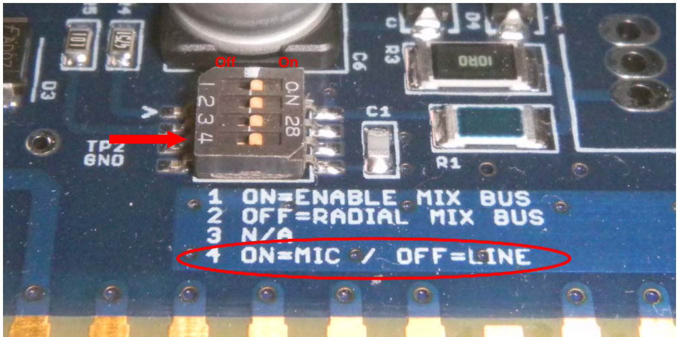
Figure 8: Line Mode Slide Switch Close-Up
