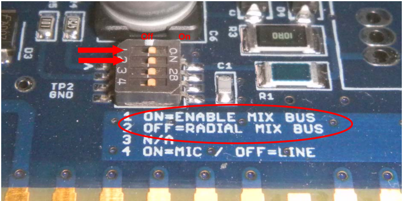
Figure 9: Slide Switch Showing Mix Buss Switch Assignment
