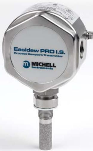
The Easidew PRO I.S. is a rugged intrinsically safe 2-wire dew-point transmitter for trace moisture measurement in liquids and gases. It is certified for use in IS Class 1 Div 1 Groups A,B,C and D, Ex II 1G EX ia IIC T4 and I.S. I 1 ABCD T4 (Ta = +60°C) hazardous area locations.
