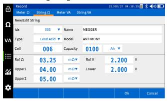
Impedance testing: measure cell impedance, voltage, and temperature
