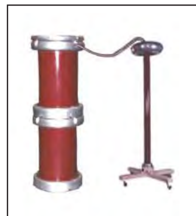
2-stage AC Voltage Test Set-up
