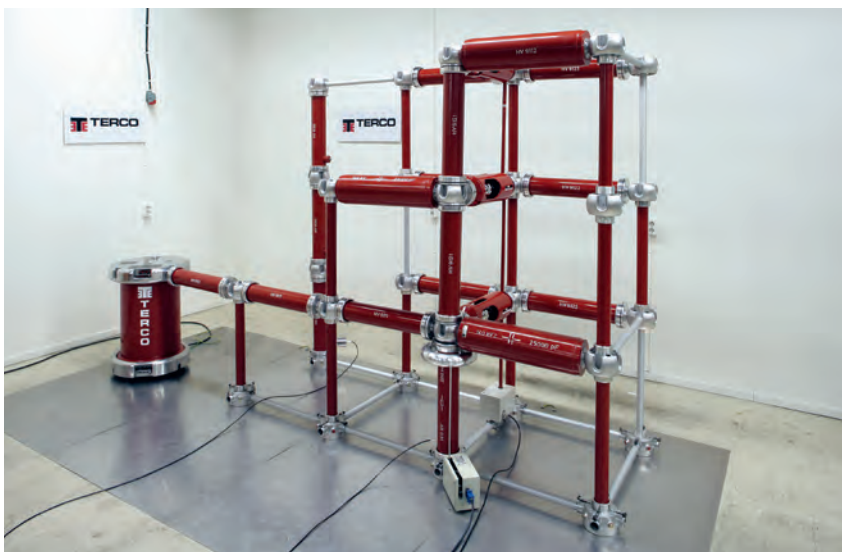
3-stage Impulse Voltage Test Set-up
