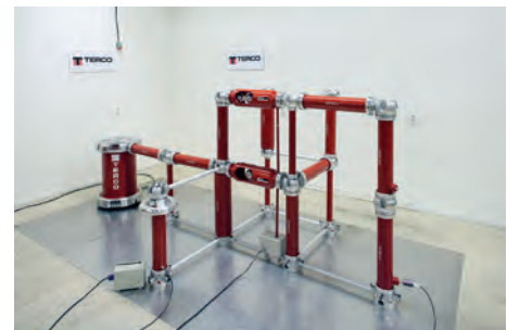
2-stage Impulse Voltage Test Set-up
