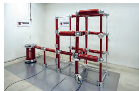
3-stage DC Voltage Test Set-up
