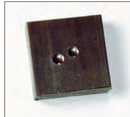
Brinell Test Piece after Brinell Indent
