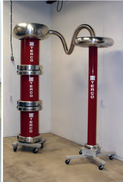
3-stage AC Voltage Test Set-up
