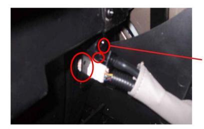
\* The air hose should be inserted into the bottom air hose opening slot shown here.
