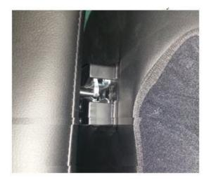
PUSH THE LEFT ARMREST FORWARD ONTO THE MAIN BODY AND UNZIP THE ARMREST COVER AND REMOVE THE CURVED BLACK PLASTIC PART SHOWN BELOW
