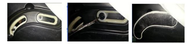
UNSCREW THE (4) SCREWS FROM THE ARMREST AND INSTALL THE REMOTE HOLDER WITH THE REMOVED SCREWS.
