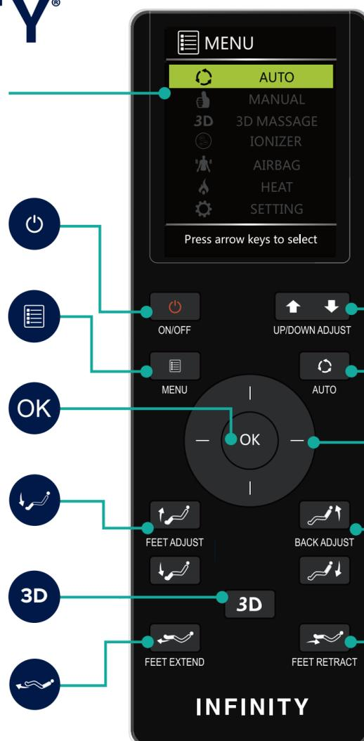
**Back Adjustment** – Back mechanism position adjustment; press and hold up to raise, press and hold down to lower. Use during initial body scan fine tuning or in manual point zone mode
