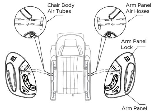
**10 Step 10:** Align the two pins on the Chair Body with the slots on the Arm Panel, making sure the air hoses are out of the way. Use your body for support to hold it in place. Re-attach the outer components of the front bushing first, then the rear. Hand screw into place.
