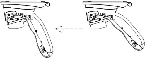
**Step 3:** Plug the remote control cord into the remote control port located on the right side of the seat cushion. Ensure the **arrows** on the top of the remote control cord and the remote control port are **lined up**. Screw on to fasten. Do not force.
