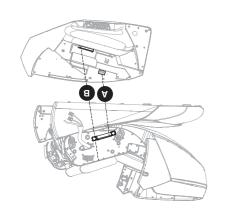
**Step 3:**Note the 2 locations each arm attaches to the chair body; locations A, and B
