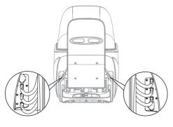
Double check that all airhose and electrical wires are still firmly connected in the back of the chair under the armrests. You can see the connections in the back of the chair, underneath the arms when fully upright.
