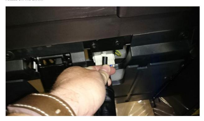
Now that power and air are connected, attach the left legrest hinge onto the body pin as show:
