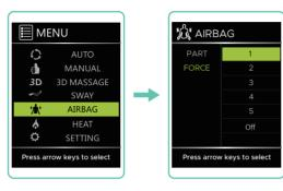
Note: Airbags must be active to set intensity level
