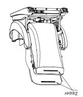
of the back of the chair body. the zipper located on the top chair body and zippering it to draping it over the top of the Attach the back cushion by Step 5:
