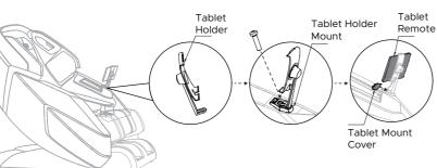
Locate the tablet holder from the accessory box. Use the screw driver to remove the two M4x12mm screws from the tablet holder mount, making sure the mount stays attached to the chair once screws are removed. Place the tablet holder into the tablet holder mount and then re-insert the two M4x12mm screws into the screw holes to secure the holder in place. Next, attach the tablet mount cover to the tablet holder mount and push into place to secure. Place the tablet remote into the tablet holder.
