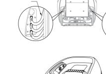
Double check that all airhose and electrical wires are still firmly connected in the back of the chair under the armrests. You can see the connections in the back of the chair, underneath the arms when fully upright.
