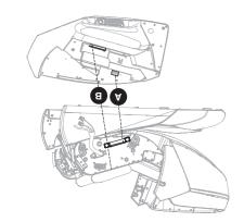
body; locations A, and B. arm attaches to the chair Note the 2 locations each Step 4:
