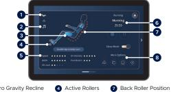
1 Zero Gravity Recline Active Rollers 2 Speakers Active 5 Indicators 8 Main Menu Navigation 3 Active Airbags 6 Time Remaining
