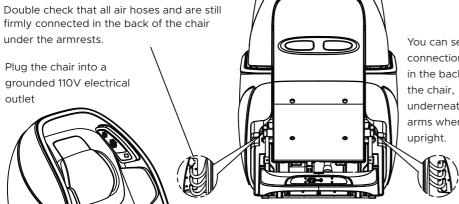
You can see the connections in the back of underneath the arms when fully
