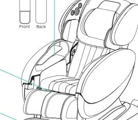
**Remote Pouch** Attach remote pouch using velcro found underneath the right arm rest
