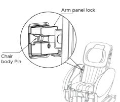
**Step 13:** Slide the metal joint pins into the opening on the chair body until the Shoulder Panel
