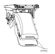
chair body. the top of the back of the it to the zipper located on the chair body and zippering draping it over the top of Attach the back cushion by Step 5:
