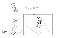
Step 7: Attach the tablet cord to the connection port on the left side of the chair seat. Be careful to line up the pins and key, then push together when aligned — do not force.
