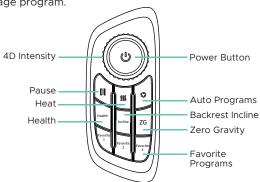
4D Intensity - Turn the dial clockwise to increase intensity and counterclockwise to decrease intensity.
