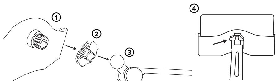
Screw the nut back onto the ball. Tighten to secure.
