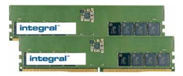
DDR5 is the latest RAM technology, engineered for next gen applications that require enhanced speed, capacity and reliability. DDR5 is 2 times faster than DDR4, 20% more energy efficient and features on-die error correction code for increased stability.
