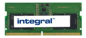
DDR5 is the latest RAM technology, engineered for next gen applications that require enhanced speed, capacity and reliability. DDR5 is 2 times faster than DDR4, 20% more energy efficient and features on-die error correction code for increased stability.
