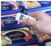
Infrared measurement in a deep-freezer
