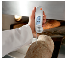
Temperature penetration measurement
