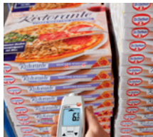
Infrared measurement in Incoming Goods
