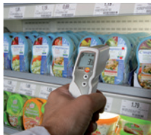
Infrared measurement refrigerated shelving
