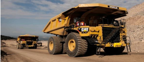
Figure 6: Autonomous Haul Trucks in The Mining Industry
