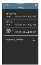
In order to pair the Bluetooth® printer with the instrument, access the "Pairing" parameter accessible via the Print menu and proceed as follows:
