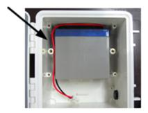
8. Re-install the battery bar. If the bar has foam on one side, make sure the foam side faces down.
