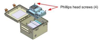
3. Use a Phillips-head screwdriver to remove the bar that secures the battery.
