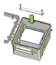
**CAUTION**: Make sure the battery cable is routed below the battery bar as shown to avoid possible shorting hazard!
