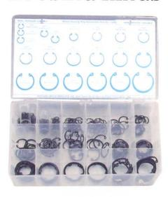
Internal, metric size rings made from spring steel with black phosphate finish have tapered design to maintain constant pressure to prevent slippage of axles, gears and bearings inside machinery housing. Meets DIN 472.
