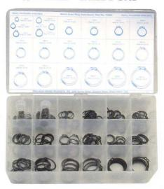
External, black phosphate coated, metric size spring steel snap rings used to retain pulleys, gears or wheels on shafts. Meets DIN 471.
