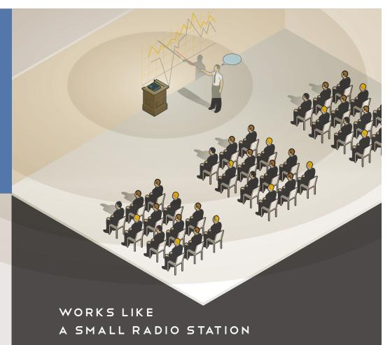
An FM listening system operates just like a small radio station. An FM transmitter, directly connected to the sound system used in a facility, broadcasts radio signals on pre-set frequencies (frequencies that the FCC has determined and restricted for use by assistive listening and language interpretation systems). These signals are received by individual "radios" – FM body-pack receivers tuned to the specific frequency used in use.
