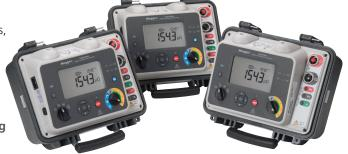
Megger has taken a no-compromise approach when designing the new DLRO100 series. The range offers a unique combination of features with everything including DualGround™ testing, adjustable current ramping, high noise immunity, high power 100 A continuous testing, and even remote control, yet still manages to be small and lightweight.
